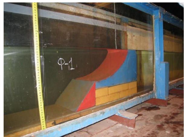
Fig. 3. A version of the design of the submerged breakwater with a steeply curved back wall of chamber that blocks the wave
