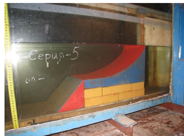
Fig. 4. A version of the design of the submerged breakwater with a gently curved rear wall of the chamber that blocks the wave
