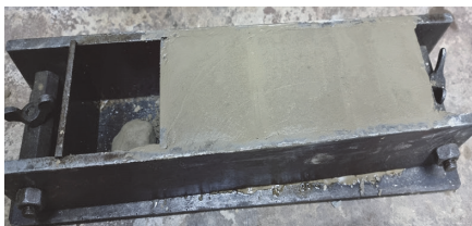
Fig. 1 – Production of 70x70x70 mm soil concrete specimens and general view
