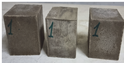
Fig. 1 – Production of 70x70x70 mm soil concrete specimens and general view
