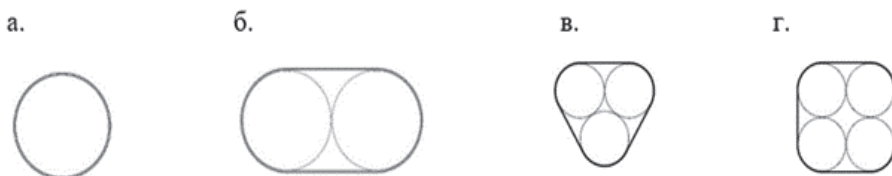
Fig.1. Structural solutions for multifunctional pipes and pipelines. Internal pipes can be made of thin steel, glass or basalt fiber
