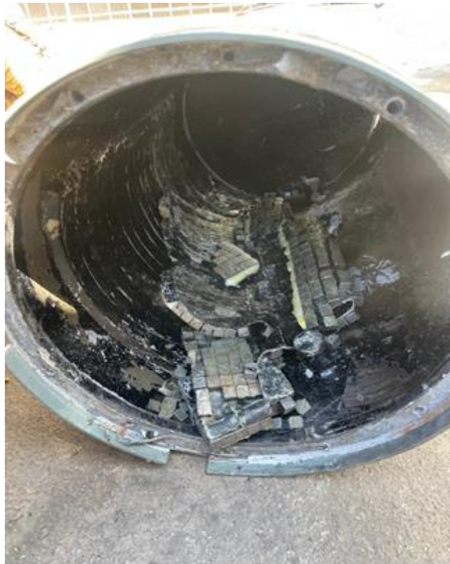
Fig. 1 The body of the undetonated missile filled with shrapnel (photo by the Denys Mykhailovskiy)
