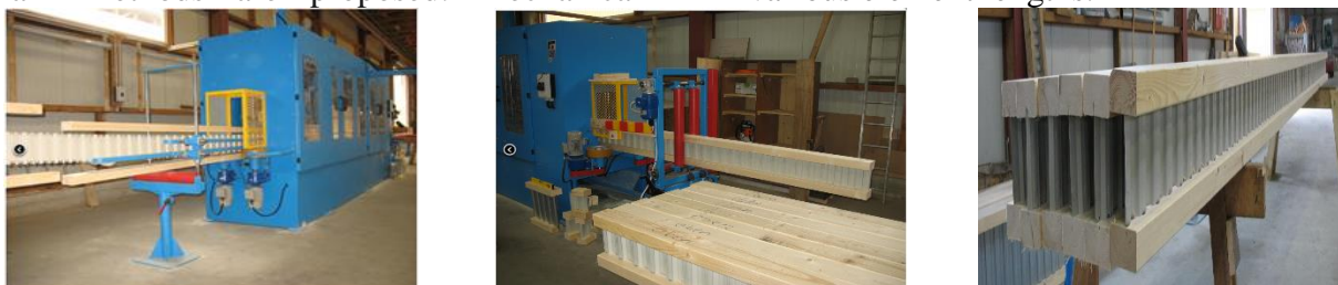
Fig. 4 The technological line for connecting steel joints with timber belts. Photo by WST Tragwerke GmbH
