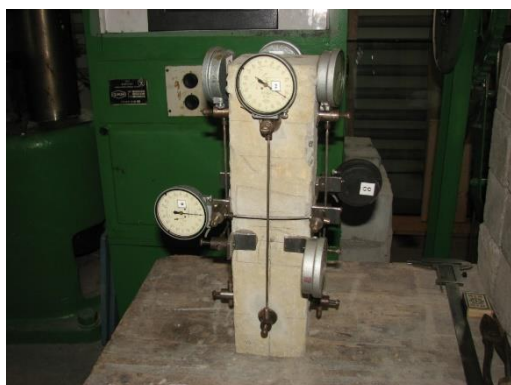
Fig.2 Installing sensors on fiber-reinforced concrete prisms. Photo by Oleg Skoruk
