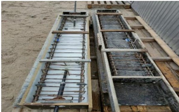
Fig. 11 Formwork and reinforcement arrangement before pouring experimental beams.
