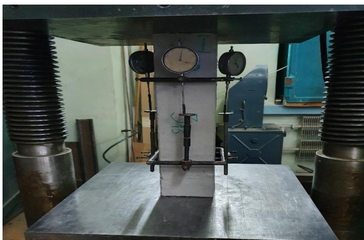
Fig 1. Determination of the deformative characteristics of concrete prisms using the P-125 press. Photo by D. Zhuk
