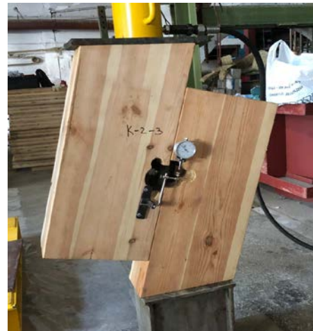
Fig. 5 Geometry of tested connection (a) and scheme of loading (b). Photo by Andrii Bidakov
