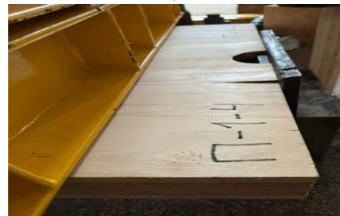
Fig. 16. Failure mode of tested specimens in series P-1: Photo by Andrii Bidakov
