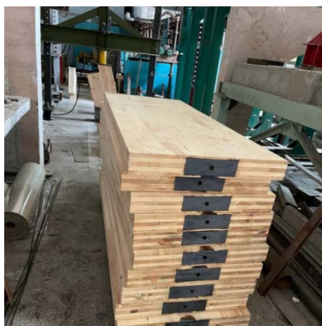
Fig. 7 Panels with connectors before tests out-of-plane. Photo by Andrii Bidakov
