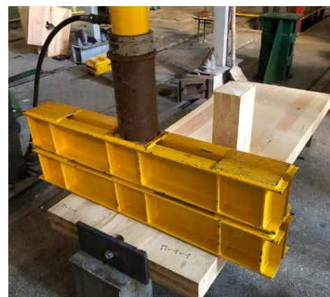
Fig. 7 Panels with connectors before tests out-of-plane. Photo by Andrii Bidakov
