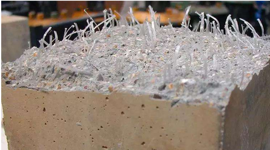
Fig. 2. Fiber concrete in section
